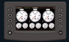
The OXE 7" display is full- featured display that integrates vital engine, transmission and diagnostic information into an easy to read operators interface. The 7" display is capable of displaying three separate engines and their respective functions, offers increased diagnostic access and data storage capability.
