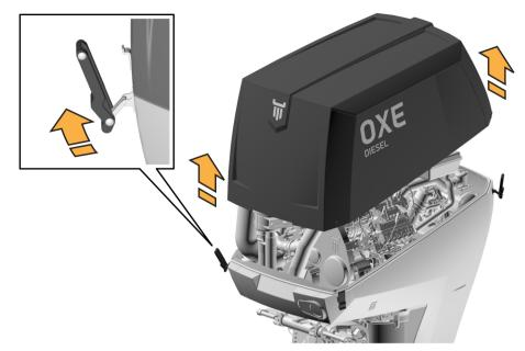
2. Before reinstalling the top cowling, check that the sealing is not dry, broken or worn, as this will allow water to enter the engine.
