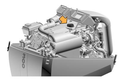
2 Remove the engine oil draining plug.
