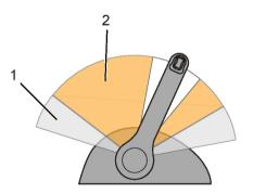
1 Full engagement propeller rpm range idle to 20% of 2 Trolling propeller rpm range: Zero to idle rpm max rpm
