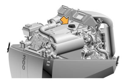
2 Check the engine oil level according to Section 2.1.5.1 "Checking the engine oil", page 21.
