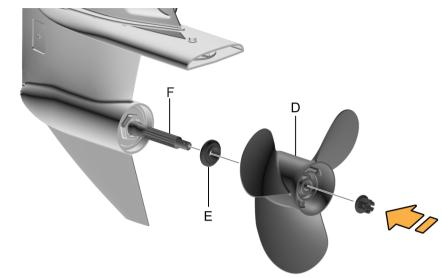
2 Install the propeller washer (E) and the propeller (D) on the propeller shaft (F).
