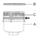
**3** Install the new oil filter cartridge.
