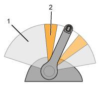
1 Normal propeller rpm range: idle to max rpm
