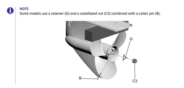
After having attached all parts and fastened the propeller nut to the correct tightening torque:
