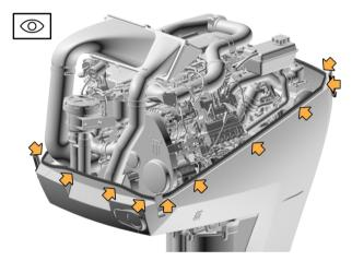
3. Lower the cowling carefully into place.
