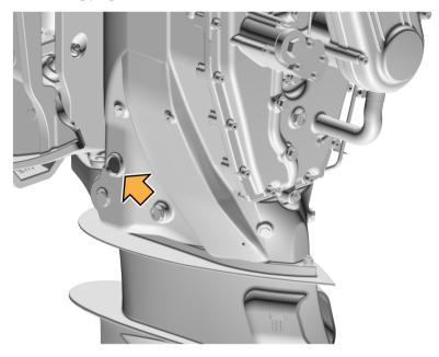
**3** Drain the engine oil into a suitable container.
