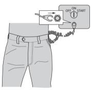
One clip must be attached to the engine shut-off switch, the other to a secure place on the operator's floating device or wrist. If the operator falls overboard or moves far enough away from the operator's position the kill-cord will stop the engine, preventing the boat from running away under power.
