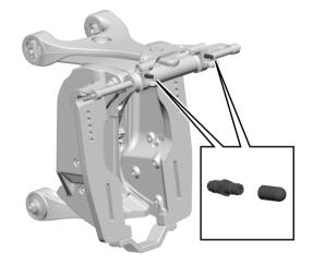
2 Fill the seatings with grease for smoother tilt operation, by applying a thin (approximately 1 mm) even coat of grease. Use grease according to Section 4.2 "Recommended fluids and grease", page 78.
