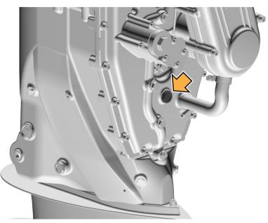
3 Fill up gearbox oil if necessary (see Section 3.8.5 "Refilling gearbox oil", page 50).
