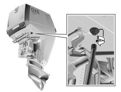
Three-way seawater drain nipple on bottom cowling
