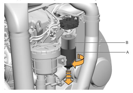
4 Insert a new 2 micron filter element (B) and reinstall the fuel filter bowl (A). Tighten by hand.
